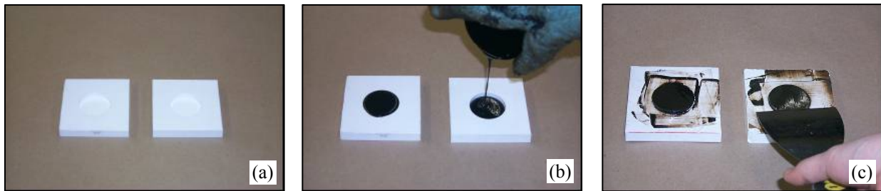
Figure M2c.1. Photo. (a) Prepare clean silicone molds. (b) Pour the molten binder. Let the binder to cool down to room temperature (approx. one hour). (c) Dress the binder with a heated putty knife (Picture by Kitae 2005).
