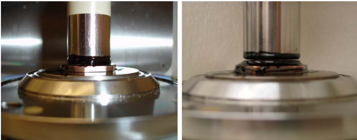
Figure E1b-1.2. Photo. Specimen before and after parallel plate tests.
